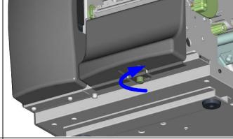
2. Open the top cover and unscrew the two screws in the front to remove the tear off bar.
