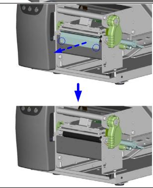
Hold the cutter and secure the cutter kit onto the printer.
