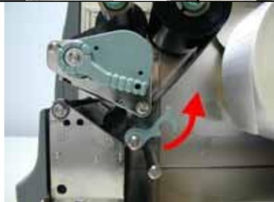
6. Feed the label through the two Label Feed Rods (under the moveable sensor) to the Tear-off Bar.
