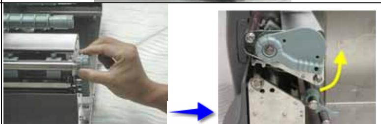
3. Take the used ribbon out of the ribbon supply shaft.
