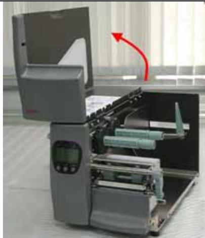
3. Pull and flip the TPH Lever counterclockwise to open the TPH.
