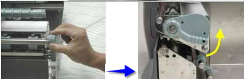
4. To remove print head, hold on to the front of the of the print head and pull it out.
