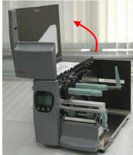
2. Flip down the Label Width Guide to make it parallel to the Label Roll Bar.
