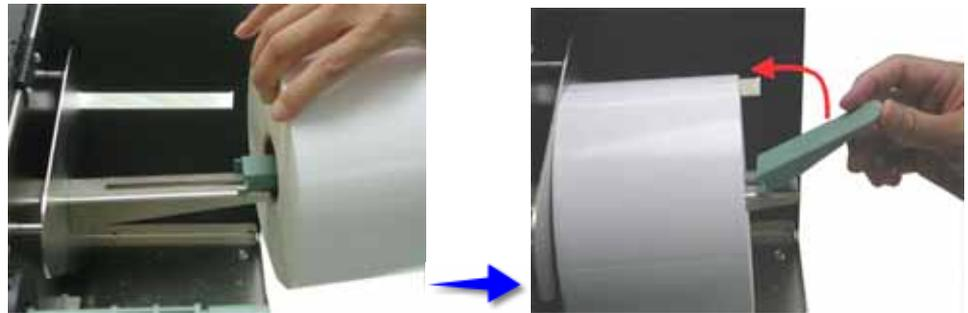
4. After the label roll is installed, push the Label Width Guide inward to secure the label roll.
