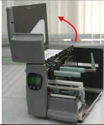
2. Pull and flip the TPH Lever counterclockwise to open the TPH.
