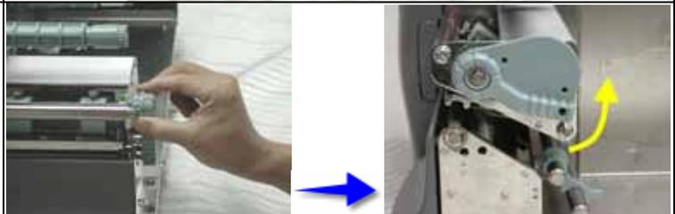
5. Flip the Label Feed Guide upward.
