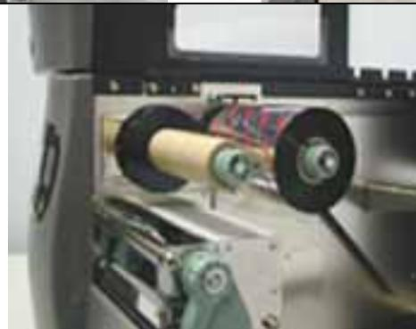
6. Feed the ribbon from the Ribbon Supply Shaft Rod under the Print Head.
