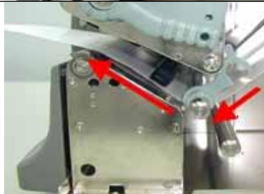
7. Align the label edge inward, and adjust the Label Feed Guide with the label.
