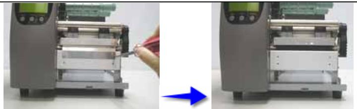
5. Hold the cutter and secure the cutter kit onto the printer.
