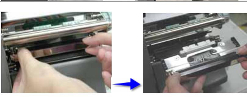
5. To install print head, hold on to the front of the print head and slide down along the track. Align the male end (with protruding pins) with the female end (pin base) and push the print head down.
