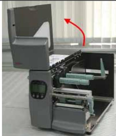
2. Place the label roll onto the Label Roll Bar, and align the label to printer's inner wall.
