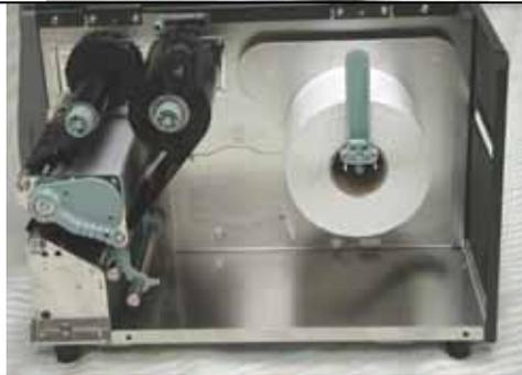
4. Pull the Print Head Lever out and flip it upward to the right.
