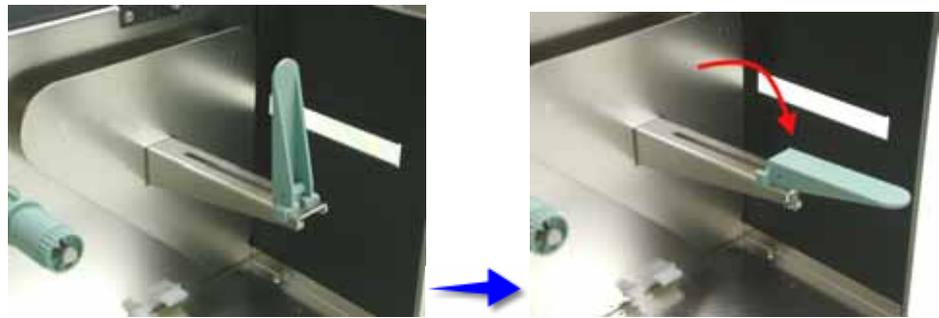
3. Place the label roll onto the Label Roll Bar, then flip back the Label Width Guide.
