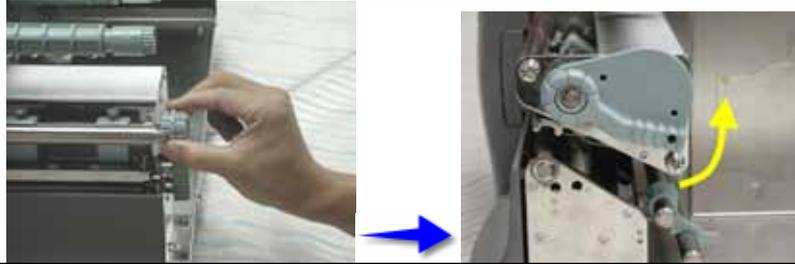
3. Use the flat tip screwdriver to loosen the TPH screws (A) on each side of the print head counterclockwise for one circle (as indicated by the arrows)
