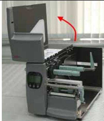
2. Pull the Print Head Lever out and flip it upward to the right.
