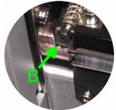
5. After the TPH print line adjustment is completed, use the flat tip screwdriver to tighten up the TPH screws (A) clockwise (as indicated by the arrows).
