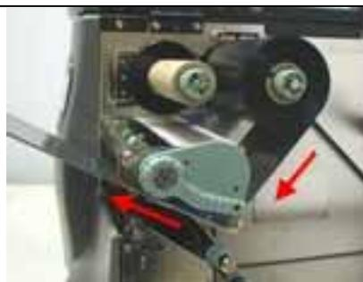
7. Wrap the ribbon around the Ribbon Shaft Rod and stick the ribbon onto the empty ribbon roll.
