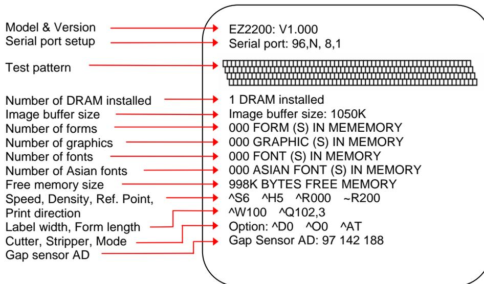
Self-Test includes the internal printer data setting.
