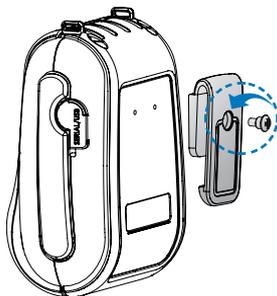
Insert the belt hook screw into the hole of the belt hook.
