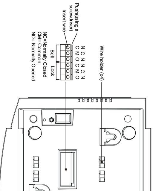
The TR40xx features two identical internal Relays with 2A switching capability (average current, peak current can be up to 10A). Relay #1 is used to control an external Bell (Ring), relay #2 controls an Electric Lock. Both normally-closed and normally-opened contacts are provided.
