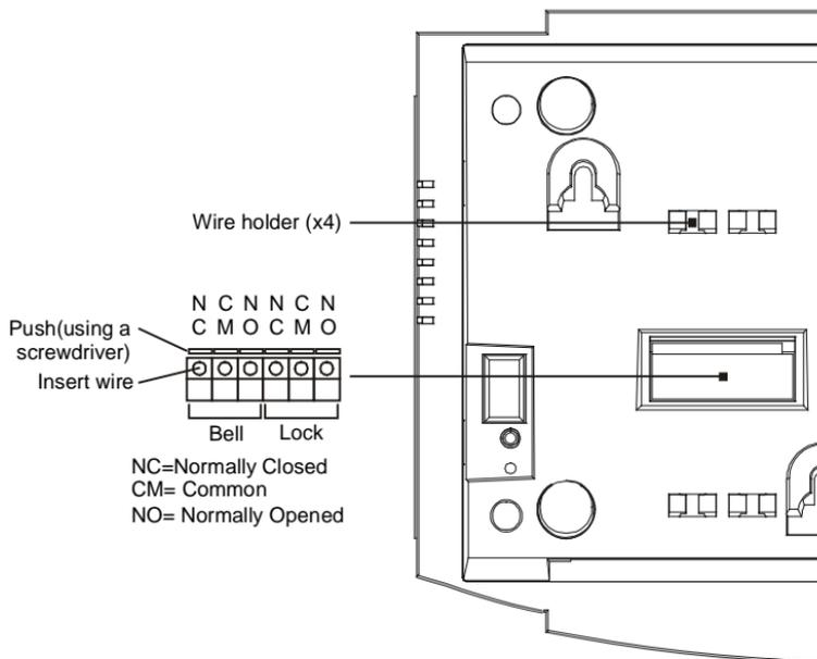
The TR4050 features two identical internal Relays with 2A switching capability (average current, peak current can be up to 10A). Relay #1 is used to control an external Bell (Ring), relay #2 controls an Electric Lock. Both normally-closed and normally-opened contacts are provided.
