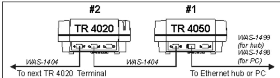
The TR4050 has a built-in TCP/IP Ethernet port so it can be placed on the Local Area Network (LAN) directly. There are two cables supplied with every TR4050: use **WAS-1499** if you want
