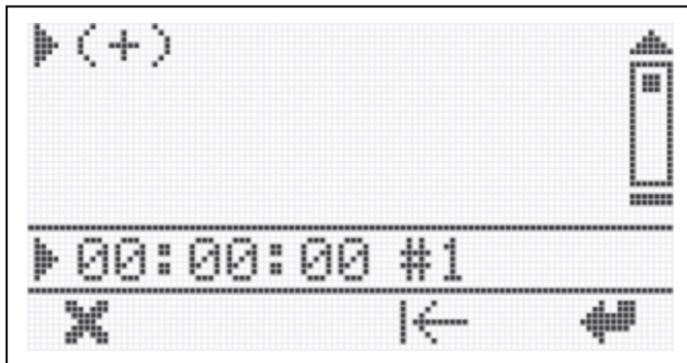
The empty table has no data records, only the “add” record prompt- (+). To add a new record, make sure that the arrow at the left of the screen points at (+) and press . The function bar will display new functions of F-keys and the edit line will display the default data for the new record (see the Figure below).
