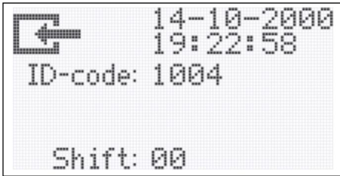
After you make sure that selected Event and Shift are correct, read the fingerprint or User ID-card (fingerprint or user Card is any working ID-card other than the Master Fingerprint or Master Card). A confirmation screen is displayed every time a new record is created. The screen shows the registered event, time and date, ID-code of the fingerprint or User Card, and the Shift (see the screenshot to the left).
