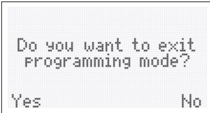
Pressing **X** when you are already at the top level of the Main Menu will prompt the TR4050 to ask you: “**Do you want to exit the Programming Mode?**” (see the Figure to the left). Notice that there are two choices displayed above the F-keys: “Yes” above the **F1** key and “No” above the **F4** key. Answer the question by pressing a desired F-key. The TR4050 displays many other messages and errors that you respond to by pressing one of the F-keys corresponding to the desired
