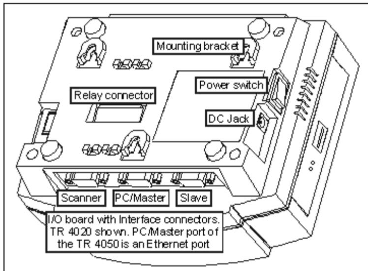
The TR4050 can be used as a wall-mount or a desktop device. You can place it on the wall using the Terminal's mounting brackets (see the Figure to the left). For desktop operation, the Terminal base can be rotated 180 degrees (to adjust the front panel's viewing angle and move away I/O connectors)- see [Rotating base cover for desktop operation](#).
