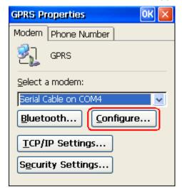
4) Select the Call Options tab. The special modem commands inserted into the dial string must be [+CGDCONT=1,,"AP name"]. For example, change "INTERNET" below to the name of your GPRS AP.
