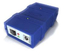
The DS100 is a Serial Device Server for external use. Device hardware includes one 10BaseT Ethernet port, one serial port and an internal processor that "glues" network and serial sides together. Internally, the DS100 is based on the <u>EM100 Ethernet Module</u>.
