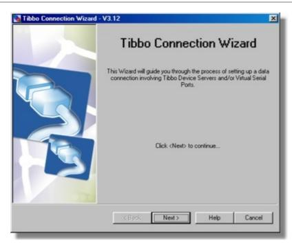
*Connection Wizard* offers a selection of jobs that help you setup several kinds of typical data links involving Tibbo Device Servers and *Virtual Serial Ports* (*VSPs*). For example, a <u>VSP-to-DS</u> job helps you create a *VSP* on the PC, and then configure this *VSP* and the Device Server (DS) of your choice to work with each other.
