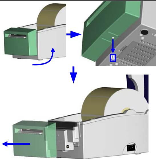
3. The adjustment screw is located on the side of the cutter. Use a screwdriver and turn the screw anticlockwise to loosen the cutter blade and pull out the jammed label.
