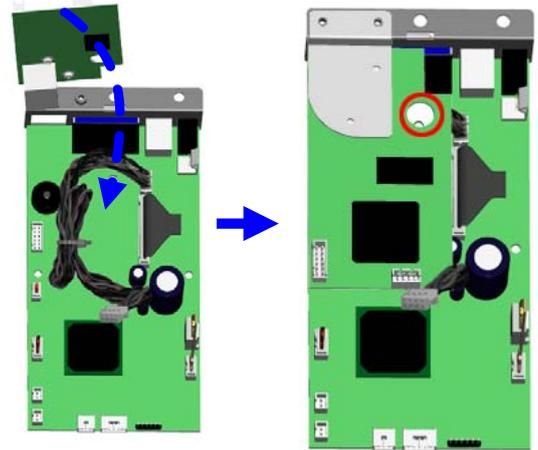
12. Secure the Ethernet module on the motherboard using the fastening screw supplied and the earthing screw.
