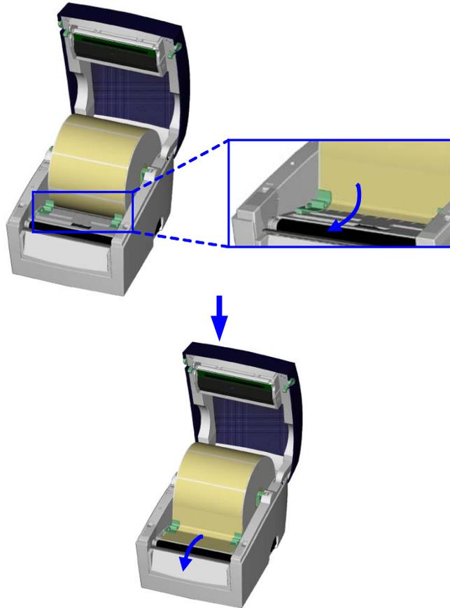
8. Adjust the paper guides to the width of the label liner.
