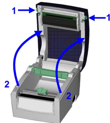
3. Place the printer the right way up again and lift the front cover.
