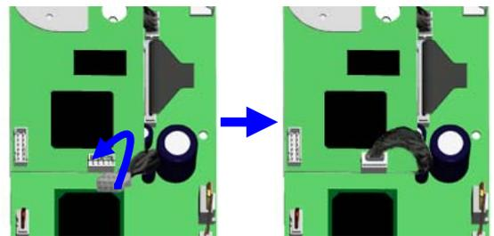
14. To avoid damage to the cable when reassembling the printer, all cables on the right of the motherboard should be routed close to the right-hand side of the housing.
