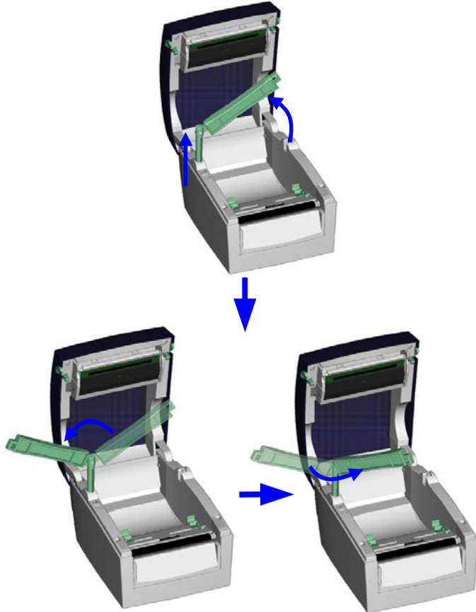
A. To load label stock with a 1" core, the locking notch must be at the top of the label supply hub.
