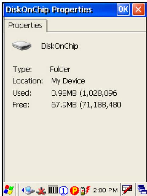
Note: The DiskOnChip is part of the onboard 128 MB flash memory. Because the flash memory is non-volatile, data or programs stored in DiskOnChip will not be erased after hardware reset.
