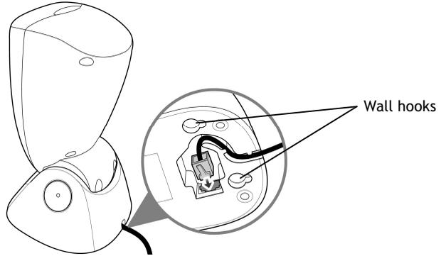
4. Align the cable through the cable hook.
