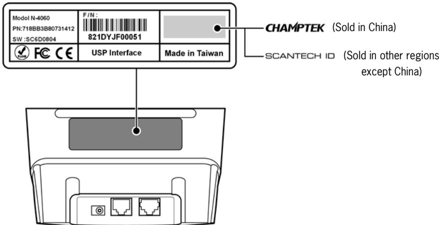
The scanner's serial number is found underneath the barcode label as depicted in the figure above. This official registration number is strictly related to the device. The supplier may ask for this number when the scanner needs servicing.
