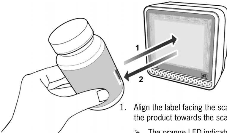
1. Align the label facing the scanner and move the product towards the scanner.
