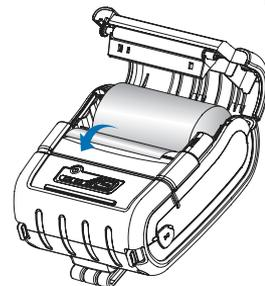
Pull a short length of paper out of the printer and close the cover.
