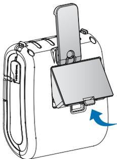
After putting up the belt clip, remove the battery holding it up as shown above.
