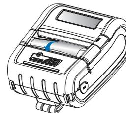
Tear off the additional paper using tear bar.
