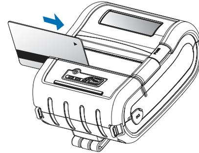
Insert and swipe the card in the direction of the arrow as shown in the picture.
