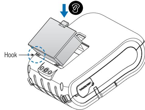
1. Align battery hook as shown in the picture
