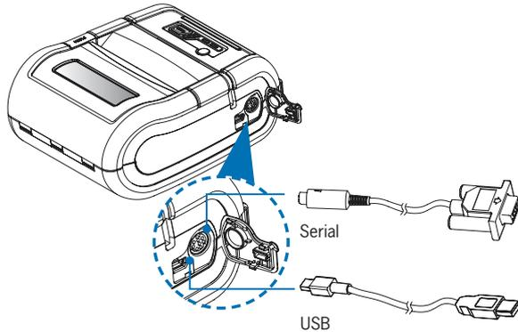
1. Connect USB or Serial cable into the cable connector on the printer.
