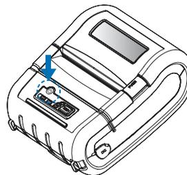
Turn off the power pressing the power button for approximately 3 seconds.
