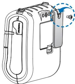
Insert the belt clip screw into the hole of Belt clip
