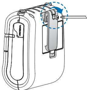
As shown in the picture, tighten the screw with a screw driver.
