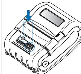
While you are pressing the FEED button, press the power button
