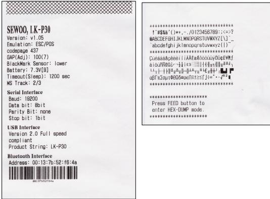
When the printer is installed initially or when you face a problem, you can run the self test and check the information about
