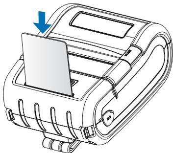
Insert the card in the direction of the arrow as shown in the picture.
