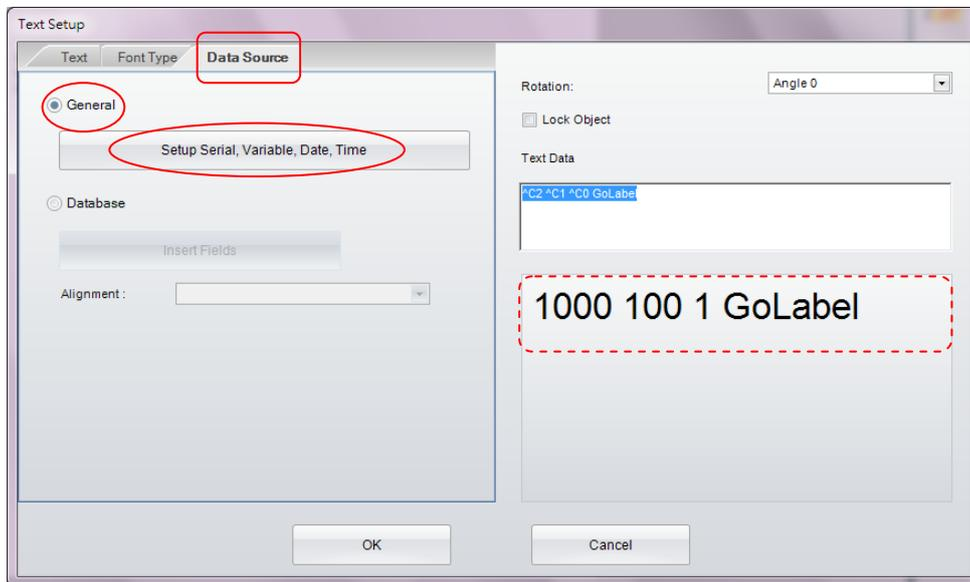
Click “Edit” in the dialog of “Setup Serial, Variable, Date, Time” to open a 4<sup>th</sup> level dialog “Serial Number Maintain”. After Editing, please select which one and click “Insert” to insert serial number to the Object.
