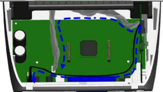
***【Caution】*** Please make sure that you position all cables in such a way that they are not damaged when you reassemble the printer.
