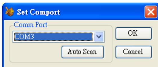
Make sure the terminal is powering on and with communication cable attached to PC. Selecting *Comm Port* where the *GuardScan* terminal is connected. Or click *Auto Scan* to detect automatically. Click *OK* to save the setting.
