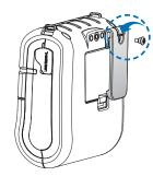
Insert the belt clip screw into the hole of Belt clip
