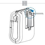
As shown in the picture, tighten the screw with a screw driver.
