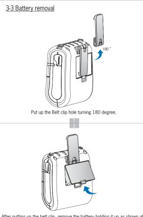
After putting up the belt clip, remove the battery holding it up as shown above.
