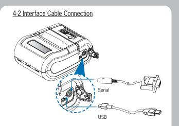
1. Connect USB or Serial cable into the cable connector on the printer.
