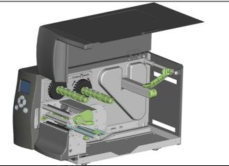
2. Pull out the print head release lever as shown in the illustration (1) and turn it anticlockwise to a top right position (2).
