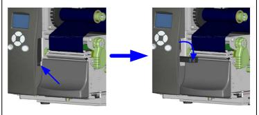
13. Close the printer cover to complete installation of the dispenser.
