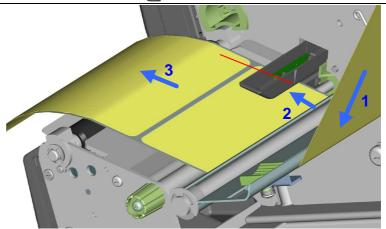
9. The labels pass between the wall of the printer housing and the adjustable paper guide.
