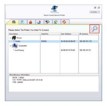
Click the magnifier icon to search the Godex printers which are connected via Ethernet port in you network environment. Once a connected Godex printer is detected, it will be listed on the start page.
