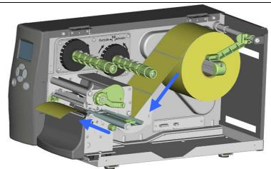
8. Pass the label stock through the sensor and up to the tear-off plate.
