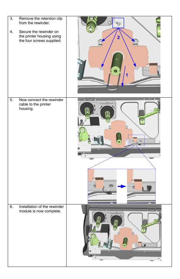
5-2. Installing the rewinder guide
