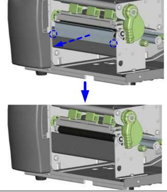
3. Secure the cutter module on the printer housing using the screws.
