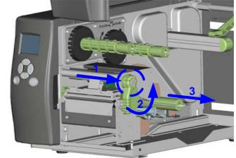
6. Now load the label roll into the printer.
