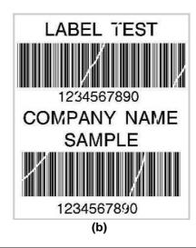
2. To keep track of the change in print quality, you should adjust the screws by half a turn at a time. Print a test page. If there is no improvement in the print result, turn the screw by another half turn. Do not turn the adjustment screw more than two full turns.
