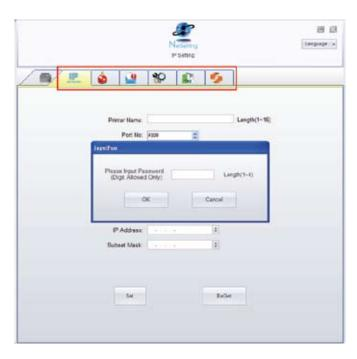
There are six tabs on the top of interface which can configure different types of network settings. But for the data security reason, you need correct password to enter the configuration pages.
