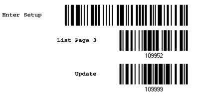
With the one-scan setup barcode #@109952#, setting is done with one scan.
