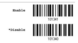
Decide whether to enable EAN-13 978 Addon Mode. When enabled, barcodes starting with **978** won't be decoded if the scanned barcodes do not have the Addon 2 or Addon 5 suffix.
