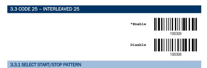
This decides the readability of all 2 of 5 symbology variants. For example, flight tickets actually use an Industrial 2 of 5 barcode but with Interleaved 2 of 5 start/stop pattern. In order to read this barcode, the start/stop pattern selection parameter of Industrial 2 of 5 should set to "Interleaved 25".
