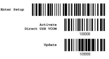
3) Read the following barcodes in sequence for the scanner to enter the download mode. The scanner will respond with beeps to indicate it is ready for downloading.
