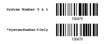
Warning: Because of the way system number 1 is encoded, if both system numbers are enabled, the user might suffer from short scanning UPC-A or EAN-13 barcodes into UPC-E1 barcodes.
