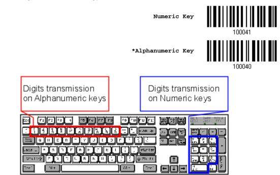
By default, the alphanumeric keypad is used for transmitting digits. Select "Numeric Keypad" if you wish to use the keys on the numeric keypad.
