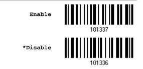
Decide whether to enable EAN-13 378/379 Addon Mode. When enabled, barcodes starting with **378/379** won't be decoded if the scanned barcodes do not have the Addon 2 or Addon 5 suffix.
