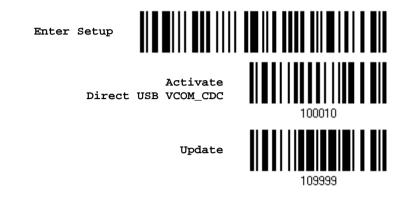
For non-Windows platform, read the following barcodes in sequence to configure the scanner to use USB Virtual COM as download interface.
