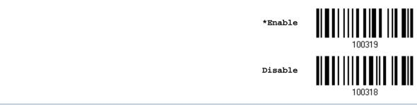
Note: When this setting is disabled, GS1-128 barcodes used to be taken as Code 128. However, starting from firmware version 1.10, GS1-128 barcodes can be decoded only when this setting is enabled.
