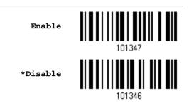
Decide whether to enable EAN-13 529 Addon Mode. When enabled, barcodes starting with **529** won't be decoded if the scanned barcodes do not have the Addon 2 or Addon 5 suffix.
