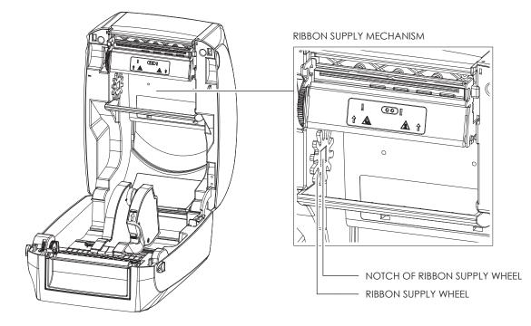
Place the ribbon supply module into the printing mechanism. Please the left-hand side of ribbon hub first. Make sure the holder of ribbon hub is inserted into the notch. Then place the right-hand side of ribbon hub.
