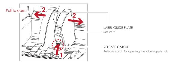
Place the label stock on label supply hubs. Make sure the label stock is aligned to both hubs. Adjust the label guide plates to fix the label width. Remember to push the release catch when moving the label guide plates.
