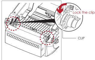
4. Close the printer cover and printing mechanism. Then to turn the printer upside down.
