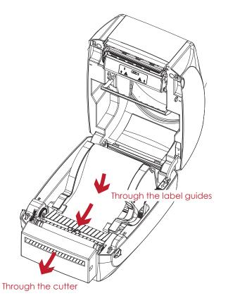
2. Close the top cover and printing mechanism. To finish, press the FEED button to set the label position.
