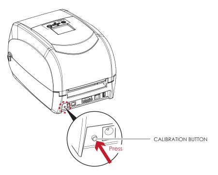
Calibration button can be used to find correct printing position or eliminate the "Media Error" problem.
