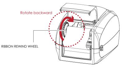
Close the cover of ribbon rewind mechanism. The ribbon loading is completed once the ribbon supply module and ribbon rewind module are assembled correctly.
