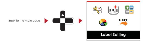
On MAIN PAGE, select the "EXIT" icon and press the FEED button to exit from SETTING MODE and the printer goes back to READY status.
