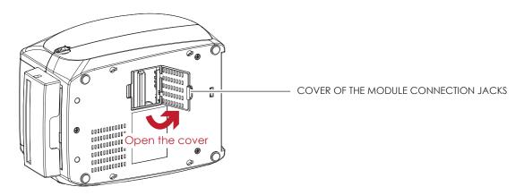
6. Plug the connector for the cutter to the jack.
