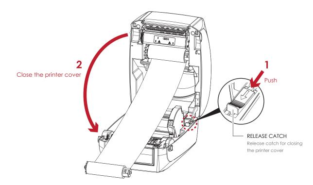
Load the Ribbon on the Printer For Ribbon Rewind Module
