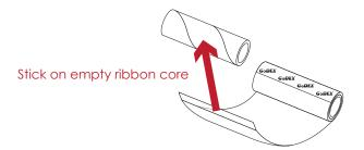
2. Insert the ribbon hub into empty ribbon core and new ribbon. Wind the ribbon around the empty ribbon core for 2 to 3 circles.
