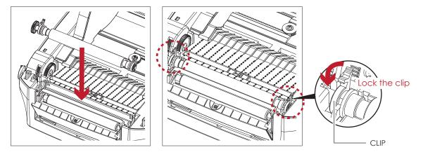
4. Close the printer cover and printing mechanism. Then to turn the printer upside down.
