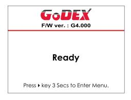
Please keep pressing • button and wait for the timer to be filled, then the LCD interface will enter into the MAIN PAGE for SETTING MODE. You can make various setting functions in SETTING MODE.
