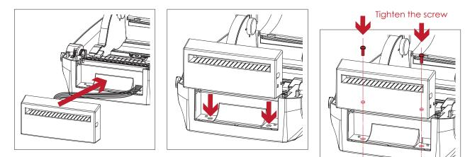
3. Place the platen back to the printer and lock the clips.
