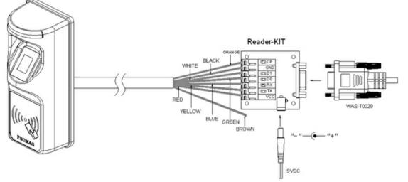
Note: MF700Kit is a test connection kit included in SmaFinger Start Kit for the purpose of configuring the reader.
